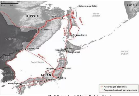
Fig. 5. Project plan of "Sakhalin-Hokkaido-Tokyo" *Source:* <u>http://edo-tokyo.livejournal.com/5796034.html</u>
