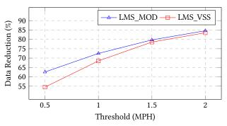
Figure 6: Data reduction for Average Wind Speed
