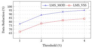
Figure 5: Data reduction for Humidity
