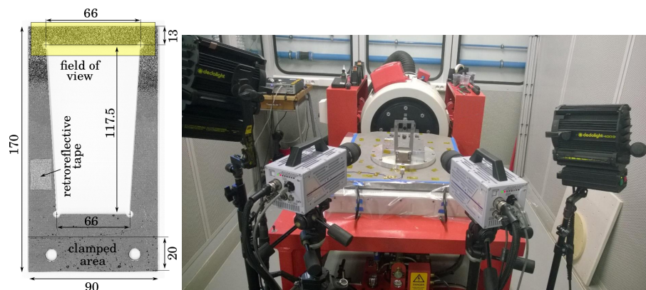
Fig. 5 Experimental setup: dimensions of the fatigue specimen (left) for the stereo case; instrumentation with two high speed cameras, two Dedolights and one single point laser vibrometer (right).
