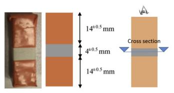
Fig. 7. Picture of isolated cement paste samples and scheme illustrating sample cuts.
