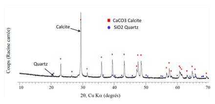
Fig. 2. Diffractogram of the limestone sample.
