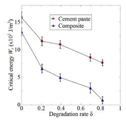
**Fig. 19.** Evolution of the critical energy as a function of the degradation rate during the shear test.
