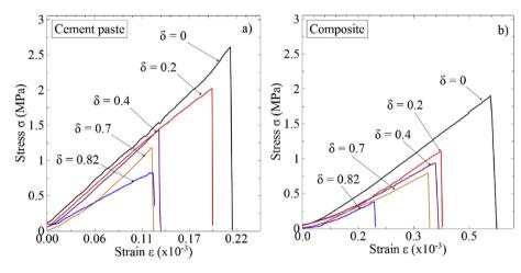
Fig. 12. Behavior in direct tensile test of sound samples and partially degraded of cement paste a) and composite b).
