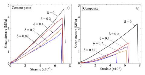
Fig. 17. Behavior in direct shear test of sound samples and partially degraded of cement paste a) and composite b).
