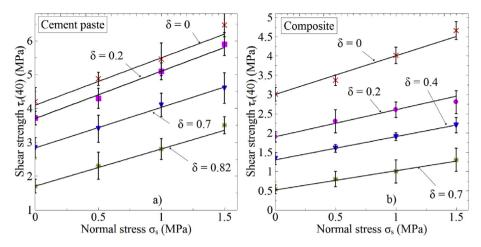
Fig. 20. Evolution of the shear strength as a function of the normal stress at different times of degradation for the cement paste a) and the composite b) at 40 days of hydration time.
