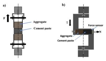
Fig. 4. Experimental devices for direct tensile test a) and direct shear test b).
