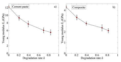
**Fig. 15.** Evolution of the Young modulus  $E_t$  as a function of the rate of degradation of cement paste a) and composite b).
