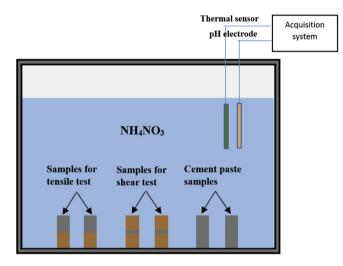
**Fig. 6.** Scheme of the leaching test of samples under ammonium nitrate solution (6 mol/l).
