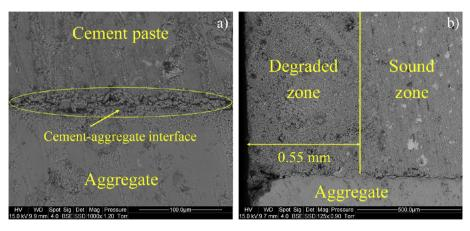
**Fig. 11.** SEM image in BSE mode of a sound sample a) and degraded after for a degradation rate of  $\delta=0.2$  b).
