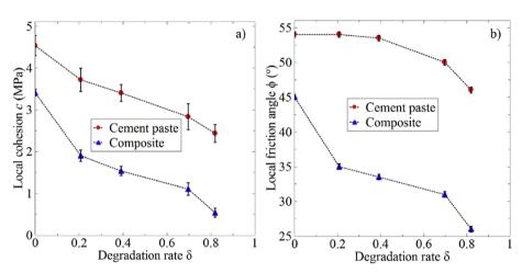
**Fig. 21.** Evolution of the local cohesion a) and local friction angle b) as a function of the degradation rate  $\delta$ .
