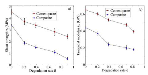
Fig. 18. Evolution of the strength  $\tau_r$  a) and tangential modulus  $E_s$  b) as a function of the degradation rate of cement paste and composite.
