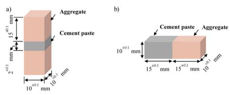
Fig. 1. Sample sizes for direct tensile tests a) and direct shear tests b).
