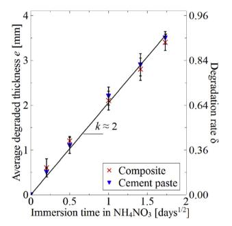
**Fig. 10.** Evolution of the degraded thickness as a function of the square root of the immersion time in ammonium nitrate.
