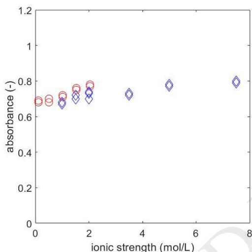
Figure 3: Influence of the ionic strength on absorbance at 353 nm.  $\diamond$ : Ionic strength change concerns the acid solution;  $\circ$ : Ionic strength change concerns the pre-mixture solution. (The interactive figure is available in the online article)
