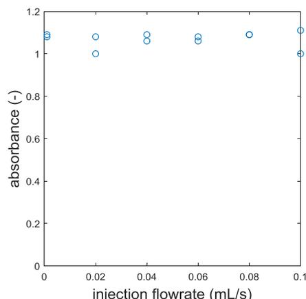
Figure 1: Influence of the injection flowrate on absorbance at 353 nm, for 2 mL of acid.  $[\text{HClO}_4] = 1 \text{ mol/L}$ ;  $[\text{H}_2\text{BO}_3^-] = 0.1 \text{ mol/L}$ ;  $[\text{KI}] = 0.0116 \text{ mol/l}$ ;  $[\text{KIO}_3] = 0.0233 \text{ mol/l}$ ;  $N = 180 \text{ rpm}$
