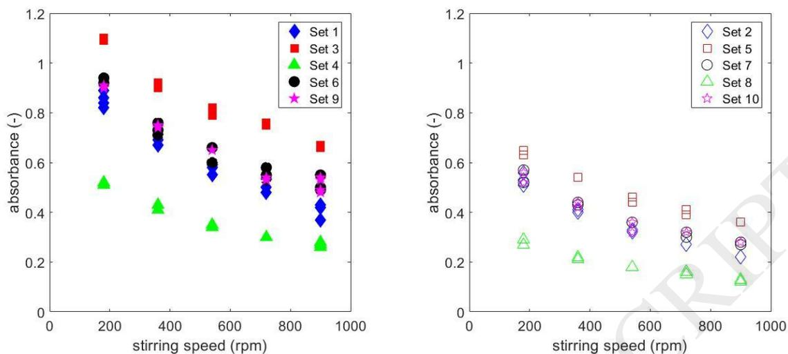
Figure 2: Influence of the stirring speed on absorbance at 353 nm, for different concentration sets using  $\text{H}_3\text{BO}_3/\text{H}_2\text{BO}_3^-$  (left) or  $\text{H}_2\text{PO}_4^-/\text{HPO}_4^{2-}$  (right). (The interactive figure is available in the online article)
