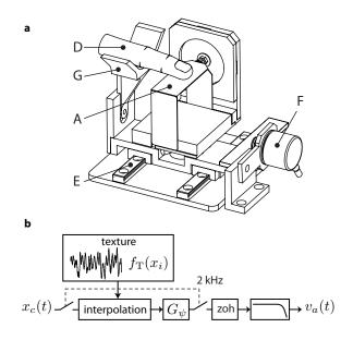
Figure 10. Stimulator operation. **a**. The transducer is mounted on linear bearing. The slider is located by an encoder. **b**. The control voltage is updated of piezoelectrical actuator as a function of the position and the texture profile used. The open loop command used.
