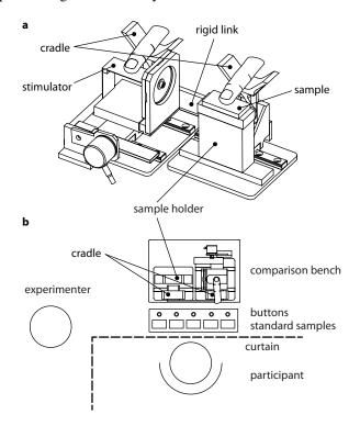
Figure 11. Experimental setup. **a**. The comparison stimuli bench. The stimulator and a real sample are side by side. During exploration, the participants experienced the stimuli under identical conditions. **b**. Participants were asked to feel the comparison texture and to match it with the standard textures. They answered by pressing one of the five buttons.
