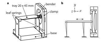
Figure 2. **a**. Transducer schematic. **b**. Cross section of the system at rest (solid lines) and during deformation (dashed lines).
