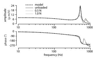
Figure 6. Frequency response of the actuator. Measurement are in grey dot and the model in plain black.
