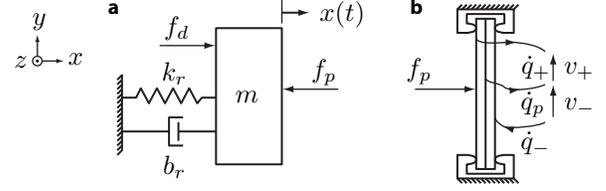
Figure 3. **a.** The plate, the sample and the bender are modeled by a mass  $m$ . It is suspended by a spring of stiffness  $k_r$  connected to a damper  $b_r$ . Forces  $f_p$  and  $f_d$  represent the piezoelectric actuator and finger interaction forces, respectively. **b.** The piezoelectric effect causes charges to appear on the electrodes as a result of displacement.
