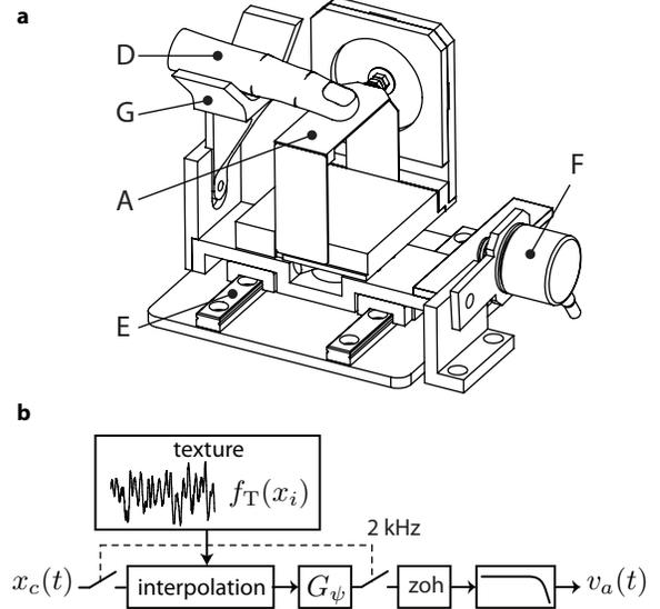
Figure 10. Stimulator operation. **a**. The transducer is mounted on linear bearing. The slider is located by an encoder. **b**. The control voltage is updated of piezoelectrical actuator as a function of the position and the texture profile used. The open loop command used.
