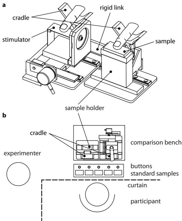
Figure 11. Experimental setup. **a.** The comparison stimuli bench. The stimulator and a real sample are side by side. During exploration, the participants experienced the stimuli under identical conditions. **b.** Participants were asked to feel the comparison texture and to match it with the standard textures. They answered by pressing one of the five buttons.
