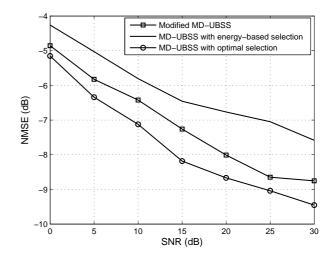
**Fig. 1.** NMSE versus SNR for 4 audio sources and 3 sensors: comparison of the performance of MD-UBSS algorithms with and without quasi-orthogonality assumption.
