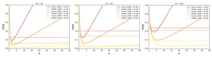
Fig. 2: Comparison of the oracle with the LMMSE for various numbers of transmit antennas and pSNRs, with respect to p.
