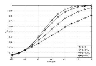
Fig. 3. Effect of  $\beta$  on the correct detection probability (M = 50).
