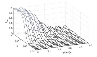
Fig. 1. Effect of  $\varepsilon$  and  $\tau$  on the correct detection probability (SNR=0 dB,  $M=50,\,P_{MS}=1+X^9+X^{11},\,N_p=8,\,P_{fa}=0.01$ ).
