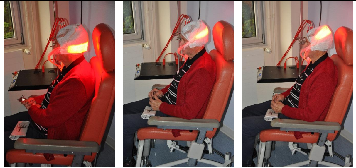
Figure 1: The three flexible light emitting textiles of the FLEXITHERALIGHT device are sequentially activated for one minute ( http://www.flexitheralight.com/ )
