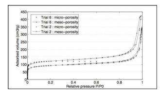
Figure 4: Adsorption/desorption isotherms of products 2 and 6 (Table 1).
