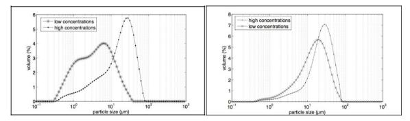
Figure 9: Particle size distributions as a function of reactants' concentrations (On the left: addition mode: parallel with mixing system and ultrasound,  $C_{MgCl2,6H2O}$ =0.81 mol/L and 1.50 mol/L, samples taken of after 210 minutes; on the right: addition mode: fast addition,  $C_{MgCl2,6H2O}$ =0.78 mol/L and 1.50 mol/L, samples taken of after 210 minutes).
