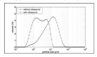
Figure 8: Particle size distributions as a function of ultrasound used during the synthesis (addition mode: parallel with mixing system,  $C_{MgCl2, 6H2O}$ =0.81 mol/L, samples taken of after 90 minutes).
