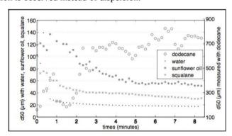
Figure 10: Disaggregation tests of a magnesium silicate (addition mode: slow addition,  $C_{MgCl2, 6H2O}$ =1.50 mol/L) in different solvents (water, sunflower oil, squalane, dodecane).
