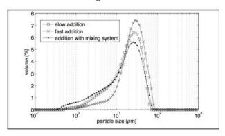
Figure 7: Particle size distributions as a function of the addition modes ( $C_{MgCl2, 6H2O}$ =1.50 mol/L, samples taken of after 90 minutes).
