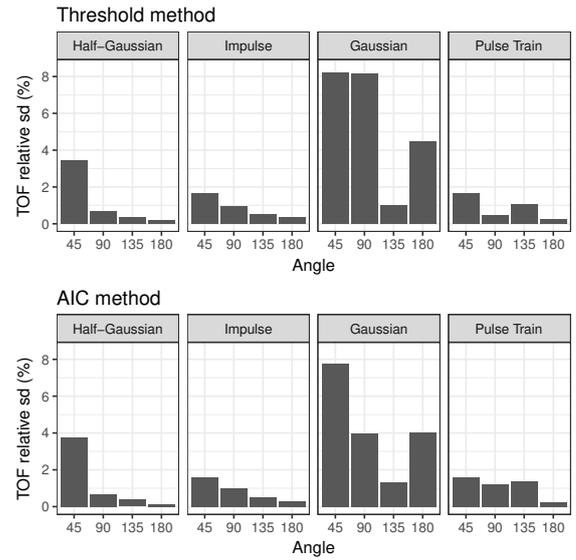
Figure 9: Relative standard deviation for TOF values using the Threshold method (up) and AIC method (down) for  $R3\alpha$ .
