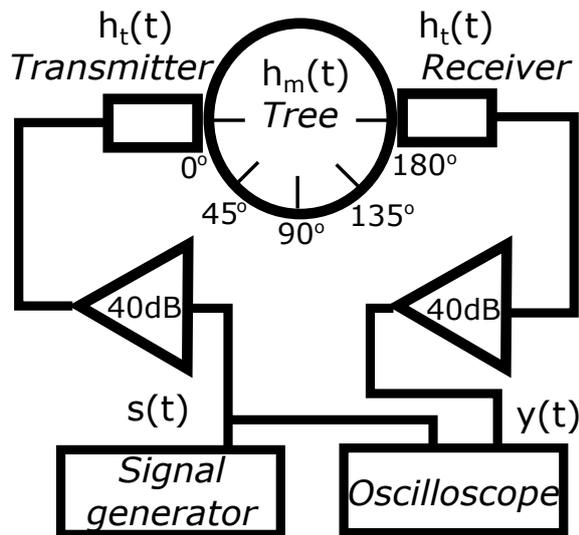
Figure 2: Ultrasonic chain for measurements.
