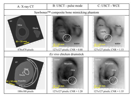
Figure 5: X-ray CT (A), USCT using an electric pulse (B), and wavelet  $\phi_{-4}(t)$  (C), of a Sawbones<sup>TM</sup> composite bone mimicking phantom (top) and an *ex vivo* chicken drumstick without skin (bottom). The white circle represents the regions involved in Contrast-to-Noise Ratio calculation.
