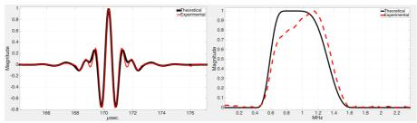
Figure 4: Time (left) and spectral (right) graph of the theoretical (black line) and the experimental (red dash line) wavelet between transmitter n°1 and receiver n°4 ( $\theta = 135^{\circ}$ ) in the absence of any object
