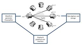
Figure 2: Electro-acoustical synoptic of the 8-parallel-channel acquisition system
