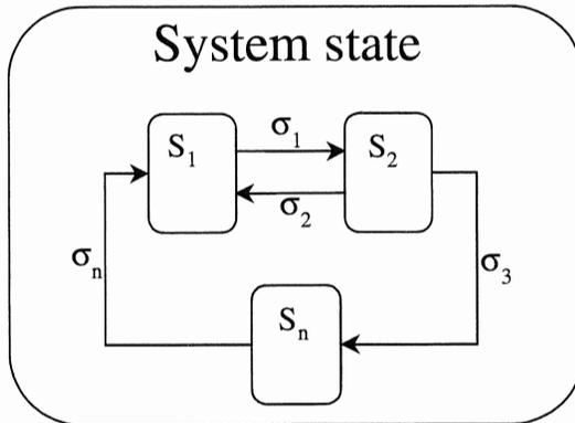
Figure 2: Partial specification Statechart showing only working modes
