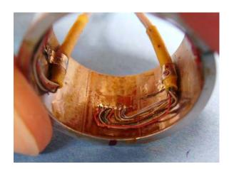
**FIGURE 2**. STRAIN MEASUREMENT ON INTERNAL ELASTIC RING WITH 45 ° STRAIN ROSETTE
