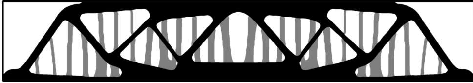
Figure 16: Test Case 10: Optimal supports with respect to the average of mechanical and thermal compliances.
