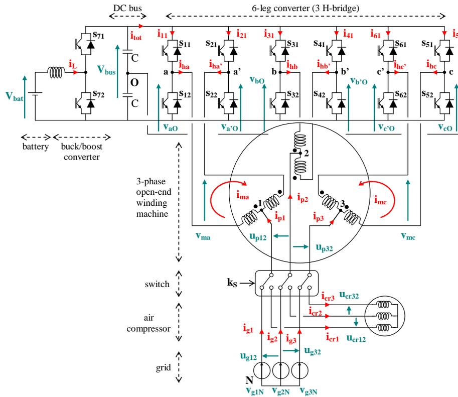
Fig. 1. The studied 3-phase open-end winding system
