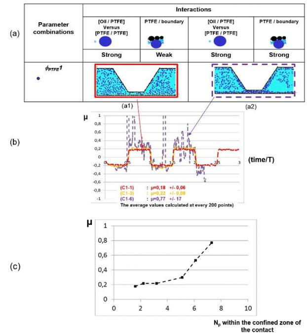
Figure 2. (a) Different tribological tendencies, (b) Evolution of the friction factor  $\mu$  for the considered combinations, (c) evolution of the friction factor  $\mu$  versus ( $N_p$ ), the number of particles within the confined zone of the contact.
