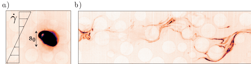
FIGURE 1. Some dye, initially confined to a small blob in a flowing particulate suspension (a), mixes with the rest of the suspension (b) by diffusing while the blob is stretched in the complex micro-flow generated by the particles.
