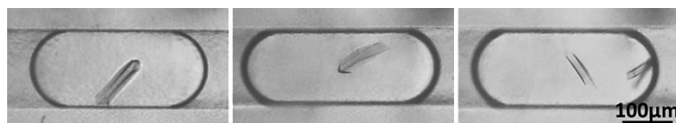
Figure 12: Pictures of 3 representative droplets for QR2 crystallization in presence of 8% DMSO in ~10nL droplets. 6.7mg.mL -1 , (NH 4 ) 2 SO 4 1.3M, 150mM NaCl, 20mM Tris-HCl pH 8, DMSO 8%, 20°C.
