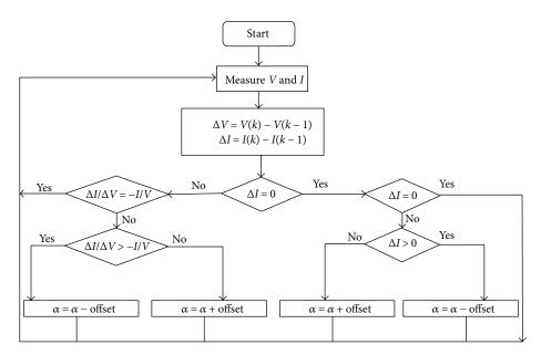
FIGURE 19: Flowchart of INC algorithm.
