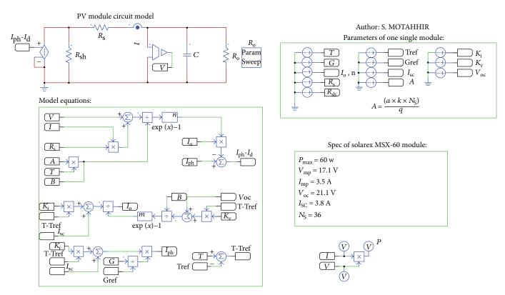
FIGURE 3: PV panel PSIM model.
