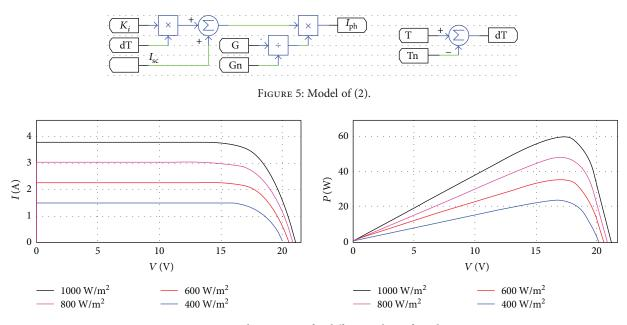
FIGURE 6: I-V and P-V curves for different values of irradiance.
