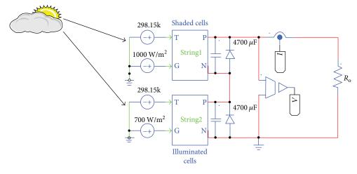
FIGURE 11: PV panel under nonuniform irradiation.
