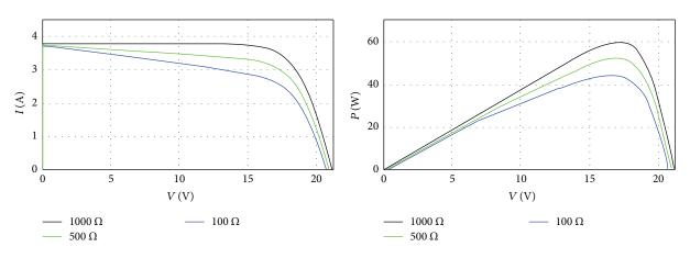
FIGURE 10: *I*-*V* and *P*-*V* curves for different values of  $R_{\rm sh}$ .
