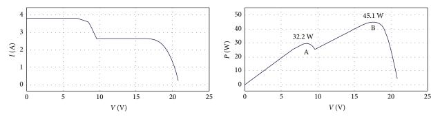
FIGURE 12: I-V and P-V characteristics of the PV panel under nonuniform irradiation.
