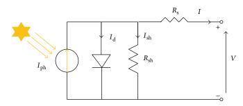
FIGURE 1: PV panel equivalent circuit.
