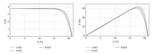
FIGURE 9: I-V and P-V curves for different values of  $R_s$ .
