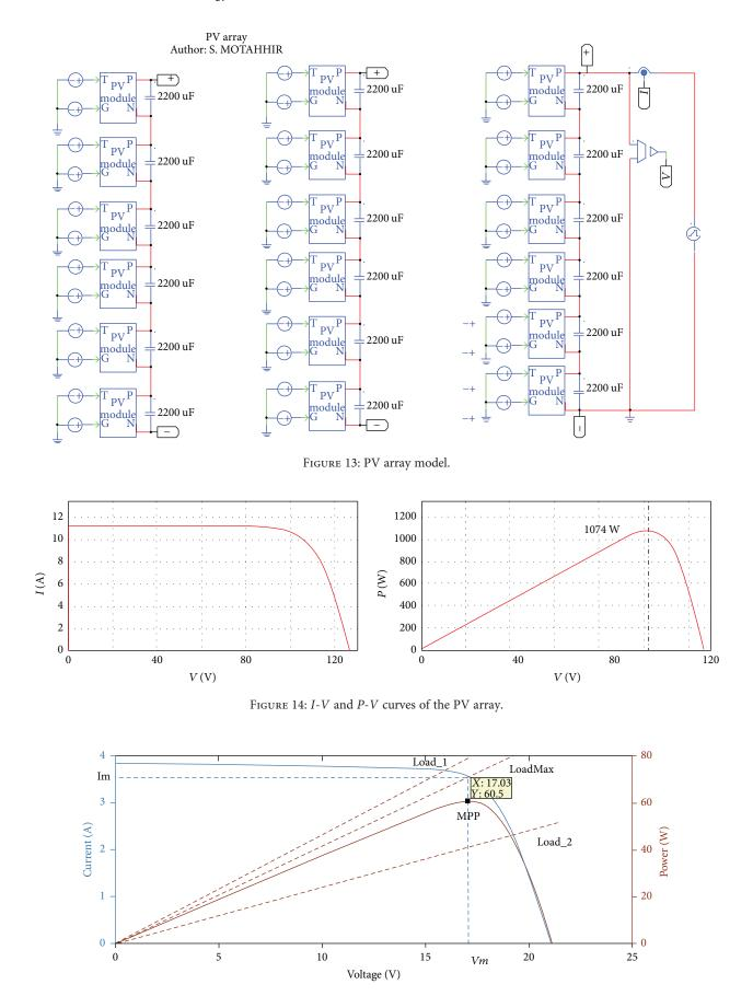
FIGURE 15: The impact of load on *I*-*V* and *P*-*V* characteristics.
