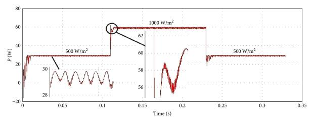
FIGURE 22: Test result of the INC algorithm.
