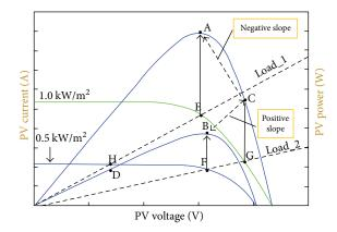
FIGURE 20: P-V and I-V curves for solar irradiation 500 W/m<sup>2</sup> and 1000 W/m<sup>2</sup>.
