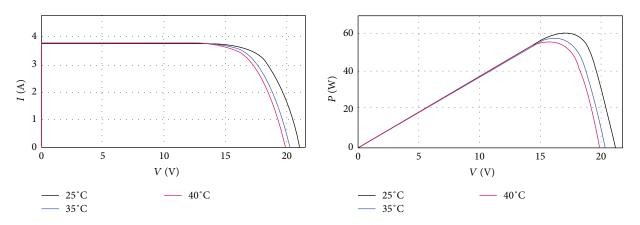
FIGURE 8: *I-V* and *P-V* curves for different values of temperature.
