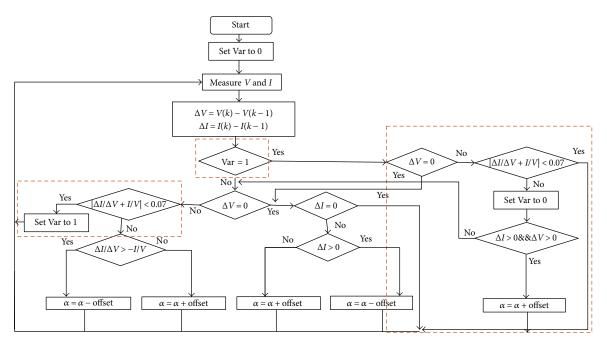
FIGURE 21: Flowchart of the proposed INC algorithm.
