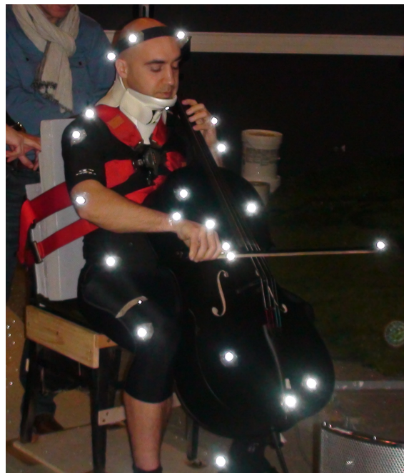
Fig. 2 Constrained postural condition in which the cellist is attached to the chair by a race harness and his head is immobilized by a collar neck. The reflective markers on the picture enable body movement recordings by motion capture cameras.
