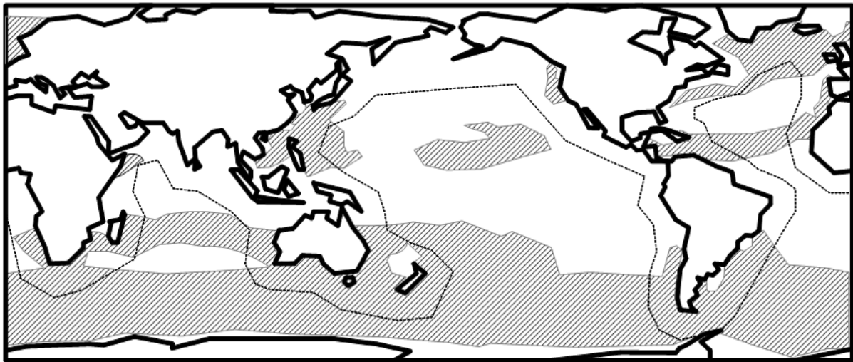
Figure 3 Offshore areas of class I wind during both the northern summer and northern winter. The dashed line indicates a distance of approximately 1,000 km to shore.
