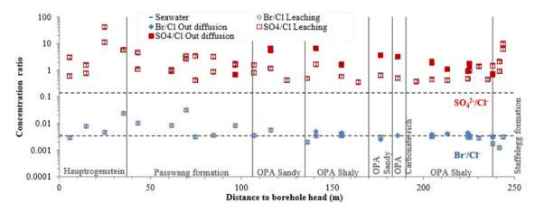
Fig. 2. Anion concentration ratios acquired by leaching and out diffusion experiments as a function of distance to BDB-1 borehole head and compared to marine ratios.
