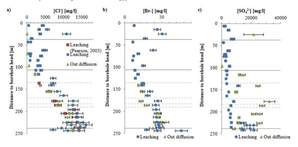
Fig. 1. Anion profiles acquired by leaching and out diffusion experiments for (a) chloride, compared to extrapolated leachate values from obtained at the tunnel level; (b) bromide; and (c) sulphate.
