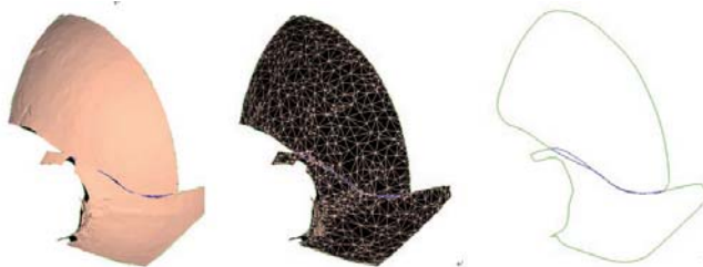
Fig. 9. Assemblage of fragment objects through contours matching meet original shape.
