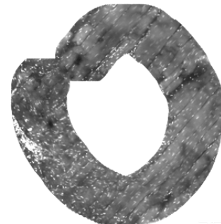
Figure 5. An open-loop real-time mosaic of a sample of chicken breast obtained with a robot circular trajectory.
