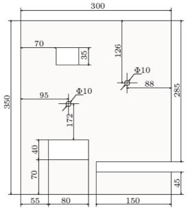
Figure 4 Dimensions of the mold
