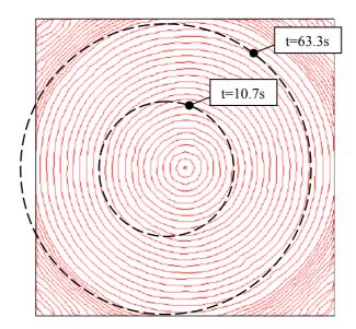
Figure 2 Filling patterns in isotropic radial injection: comparison with analytical solution
