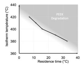
Figure 2. PEEK Processing window
