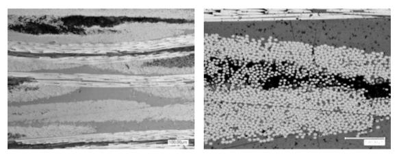
Figure 11. Film stacking microstructure after 10 minutes at 400°Cwith a consolidation pressure of 8 bars
