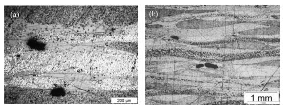
**Figure 9.** Microstructure of commingled NCF (a) 5 minutes at 420°C (b) 20 minutes at 380°C
