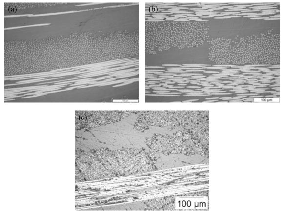
**Figure 7.** Microstructure of powdered fabric laminates (a) 5 minutes at 420°C (b) 20 minutes at 380°C (c) 10 minutes at 380°C
