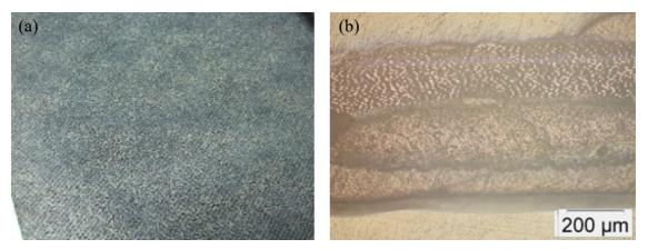
Figure 3. Powdered fabric from Porcher Composites (a) surface aspect (b) thickness microstructure
