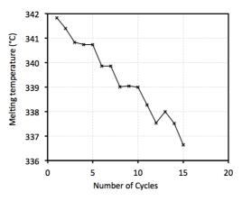
Figure 6. Influence of heating and cooling cycles on the melt temperature of PEEK
