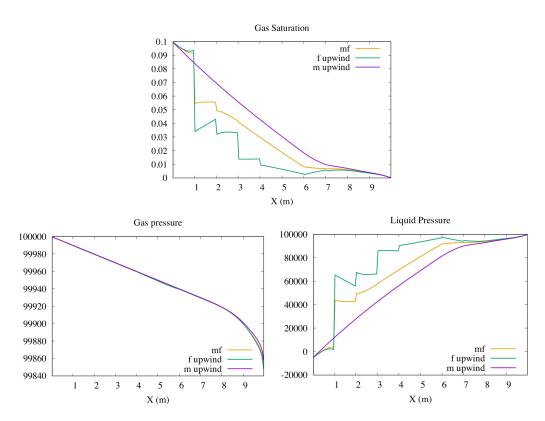
Figure 14: Cuts at x = 7.5 m of the gas saturation (top), water pressure (left bottom) and gas pressure (right bottom) at final simulation time for the hybrid-dimensional models.
