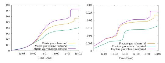
Figure 13: Gas volume in the matrix and in the fracture network as a function of time for the hybrid-dimensional models.
