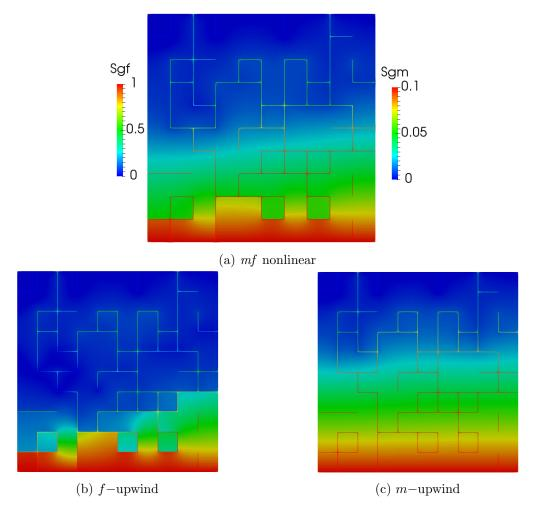
Figure 12: Gas saturation at final time computed by the hybrid-dimensional models for the desaturation by suction test case.
