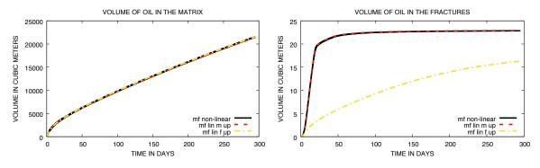
Figure 17: Comparison of the matrix and fracture volumes occupied by oil as a function of time for the different models.
