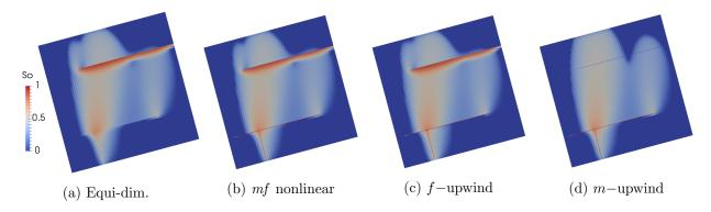
Figure 11: From left to right, oil saturation at final time computed by the equi-dimensional and hybrid-dimensional models for the three drains and one barrier test case.
