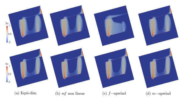
Figure 6: From left to right: oil saturation at final time for the equi-dimensional and hybrid-dimensional models. Top row: Cartesian mesh of size  $68 \times 72$  for the equi-dimensional model and of size  $64 \times 64$  for the hybrid-dimensional models. Bottom row: Cartesian mesh of size  $260 \times 264$  for the equi-dimensional model and of size  $256 \times 256$  for the hybrid-dimensional models.
