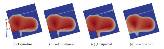
Figure 9: From left to right: oil saturation at final time computed by the equi-dimensional and hybrid-dimensional models for the viscous dominant test case with overpressure of 2.  $10^6$  Pa
