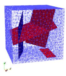
Figure 15: Geometry of the domain  $\Omega = 100 \text{m} \times 100 \text{m} \times 100$  m with the fracture network in red (left), coarsest tetrahedral mesh with 47670 cells (right).
