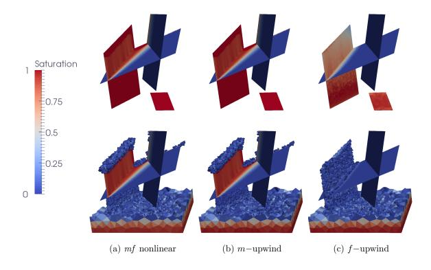
Figure 16: Comparison of the oil saturation at time t=295 days for the hybrid-dimensional models using a matrix oil saturation threshold at 0.01. Upper line: fracture network only.
