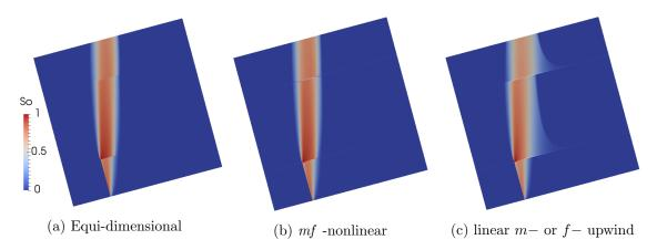
Figure 4: Oil saturation at final time computed by the equi-dimensional and hybrid-dimensional models for the gravity dominant test case with homogeneous capillary pressures. The mesh is Cartesian of size  $260 \times 264$  for the equi-dimensional model and of size  $256 \times 256$  for the hybrid-dimensional models.
