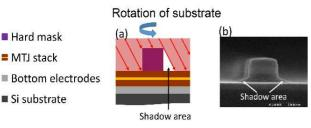
Fig. 1. (a) Conventional IBE process for the patterning of MTJ pillars. The material is etched at an angle to minimize redeposition on MgO sidewalls but this leads to shadowing effect yielding tapered sidewalls. (b) SEM image of a MTJ pillar patterned by IBE process.
