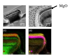
Fig.10. Cross sectional TEM (a, b) and chemical analysis (c,d) of the MTJ stack deposited on 200 nm pre-patterned Ta pillars.
