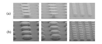
Fig. 7. Side view SEM images of arrays of pre-patterned Ta pillars of various diameters, (a) Before and (b) After MTJ stack deposition. One can clearly distinguish the material deposited on top of the pillars and in the spaces between them.
