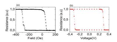
Fig.14. (a) Room temperature magnetoresistance loop of perpendicular MTJ stack deposited on pre-patterned Ta/Pt pillars versus (a) perpendicular magnetic field and (b) voltage.
