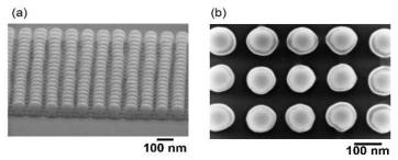
Fig. 8. SEM images of F=80 nm diameter of extremely dense MTJs arrays (pitch=1.5F) deposited on pre-patterned Ta/Pt posts: (a) Side view and (b) Top view.
