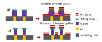
Fig.2: Illustration of the importance to pattern the non-magnetic conducting posts with undercut or V-shape. a) After depositing the MTJ material on posts without undercut, neighboring pillars are electrically interconnected due to metallic deposits at the foot of the posts. (b) When posts with undercut are used, no metallic material is deposited at the foot of the posts thus allowing good electrical separation between all pillars.
