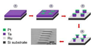
Fig. 3. Fabrication process of undercut Ta pillar using RIE. Typical SEM image of the undercut Ta pillars on Si wafer after RIE etching process.
