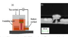
Fig. 13. (a) Illustration of MTJ stack on Ta post with electrical contacts for transport measurements. To electrically contact the MTJs, the trenches between the pillars were filled with a planarizing resist ACCUFLO. This step was followed by a resist etch-back process to open the top contact and by the patterning of the top contacting electrodes. The contacted devices were then electrically characterized (b) SEM cross section view of a device for electrical test.
