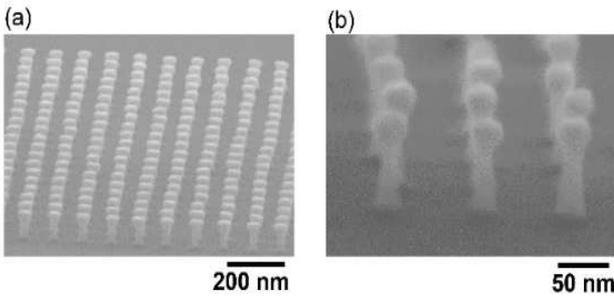
Fig. 5. SEM images of very dense array of Ta posts with undercut: Diameter of 50 nm (a) and 35 nm (b). Fig. 5b shows dense arrays of posts of size below 35 nm exhibiting a controlled 5 nm undercut
