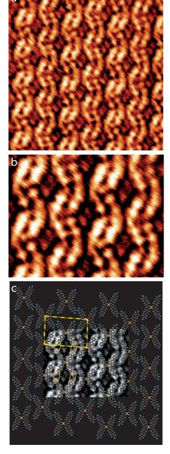
Figure 5: High resolution STM images of the complex-2 self-assembled porous network, (a)  $15 \times 15 \text{ nm}^2$ ,  $V_s = 0.95 \text{ V}$ ,  $I_t = 9 \text{ pA}$ , (b)  $8 \times 6 \text{ nm}^2$ ,  $V_s = 0.95 \text{ V}$ ,  $I_t = 9 \text{ pA}$ . (c) Assembly model with the STM image in (b) placed underneath as a guide for the eyes.  $X_2$  synthons are highlighted with orange ellipses.
