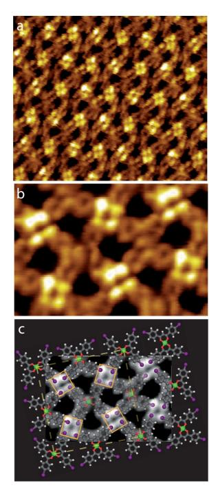
Figure 3: High resolution STM images of the complex-1 self-assembled porous network, (a)  $10 \times 8 \text{ nm}^2$ ,  $V_s = 0.95 \text{ V}$ ,  $I_t = 9 \text{ pA}$ , (b)  $5 \times 3 \text{ nm}^2$ ,  $V_s = 0.95 \text{ V}$ ,  $I_t = 9 \text{ pA}$ . (c) Assembly model with the STM image in (b) placed underneath as a guide for the eyes.  $X_4$  synthons are highlighted with orange squares.
