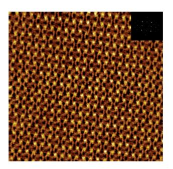
Figure 2: STM image of the complex-1 self-assembled porous network at the 1-phenyloctane/graphite interface,  $35 \times 35$  nm<sup>2</sup>,  $V_s = 0.55$  V,  $I_t = 9$  pA. Inset: FFT of the STM image.
