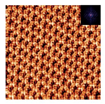
Figure 4: STM image of the complex-2 self-assembled porous network at the 1-phenyloctane/graphite interface,  $27 \times 27$  nm<sup>2</sup>,  $V_s = 0.95$  V,  $I_t = 9$  pA. Inset: FFT of the STM image.
