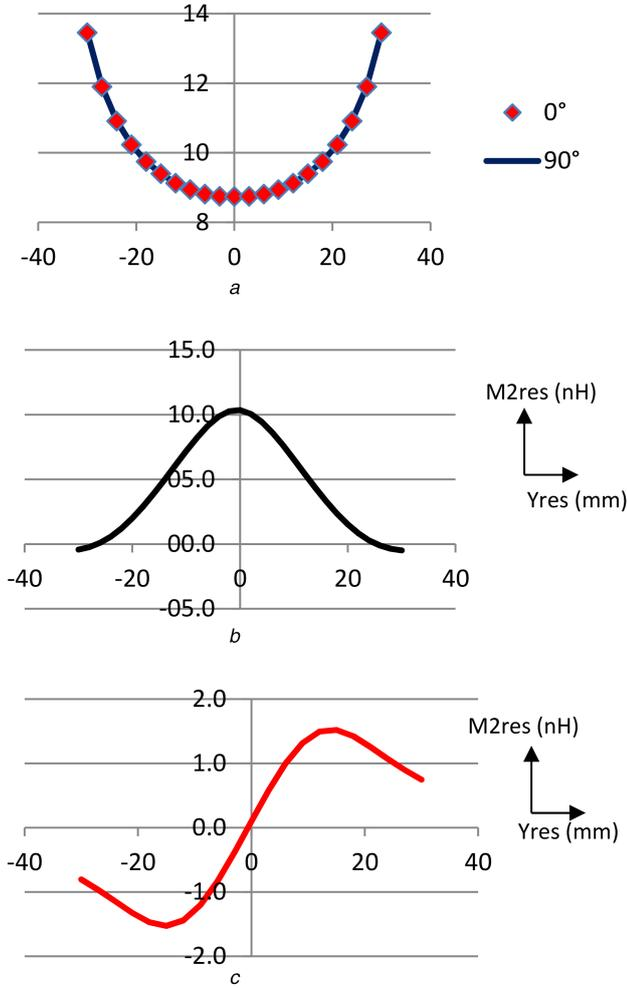
**Fig. 3** The mutual inductances ( $M_{1res}$ ) and ( $M_{2res}$ ) for different resonator positioning ( $-30 \text{ mm} < Y_{res} < 30 \text{ mm}$ ) (a) ( $M_{1res}$ ) between the reader coil and the resonator, (b) ( $M_{2res}$ ) between the tag coil and the resonator in parallel configuration and (c) ( $M_{2res}$ ) between the tag coil and the resonator in perpendicular configuration for different resonator positioning ( $-30 \text{ mm} < Y_{res} < 30 \text{ mm}$ )
