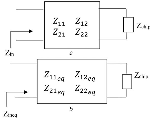
**Fig. 5** Equivalent electrical circuit of RFID system
