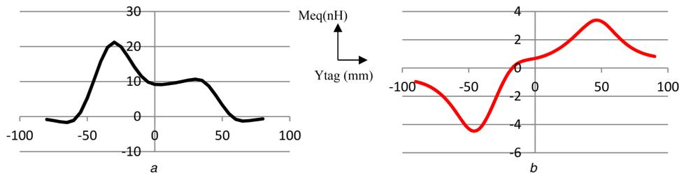
**Fig. 4** Equivalent mutual inductance ( $M_{eq}$ ) between the reader coil including one resonator (positioned at  $Y_{res} = -30 \text{ mm}$ ) and the tag coil, respectively, in (a) Parallel configuration, (b) Perpendicular configuration for tag misalignment: from ( $Y_{tag} = -100 \text{ mm}$ ) to ( $Y_{tag} = 100 \text{ mm}$ )
