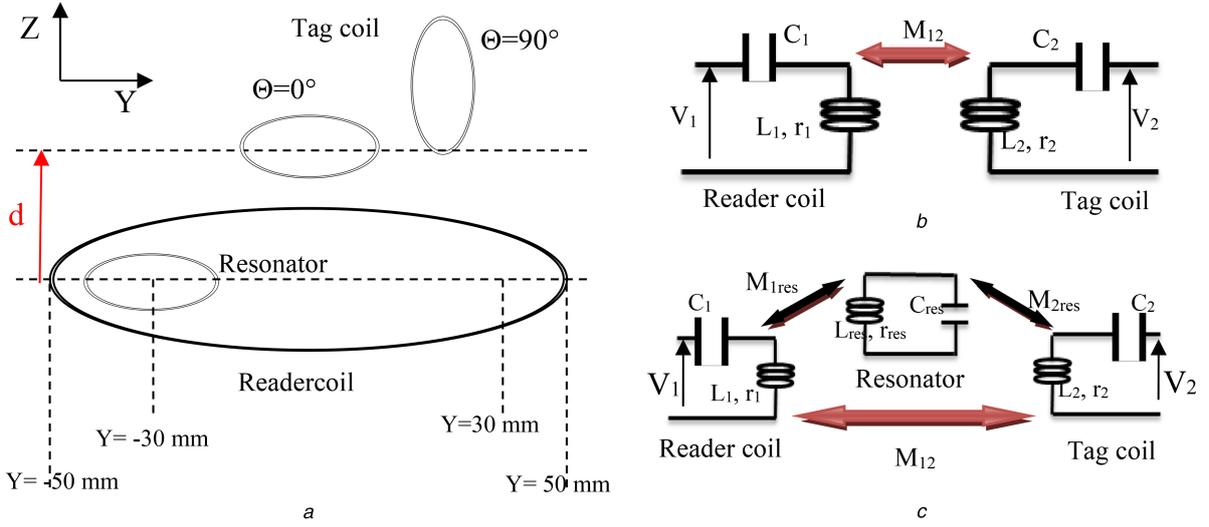
**Fig. 1** Proposed reader coil including (a) One resonator, (b) Its electrical model without resonator, (c) Its electrical model with resonator
