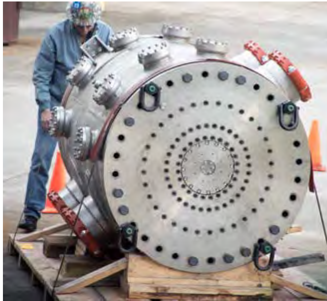
Fig. 20. Photograph of the 41.4 T resistive magnet at the NHMFL-Tallahassee (August 2017). This magnet has a 32 mm bore and is powered with a 32 MW power supply. Its design is based on Florida-Bitter plates (see text) using high-strength copper-silver-alloy conductor. Photo courtesy of the NHFML-Tallahassee.
