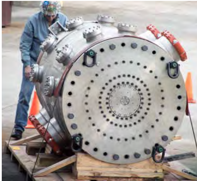
Fig. 20. Photograph of the 41.4 T resistive magnet at the NHMFL-Tallahassee (August 2017). This magnet has a 32 mm bore and is powered with a 32 MW power supply. Its design is based on Florida-Bitter plates (see text) using high-strength copper-silver-alloy conductor. Photo courtesy of the NHMFL-Tallahassee.
