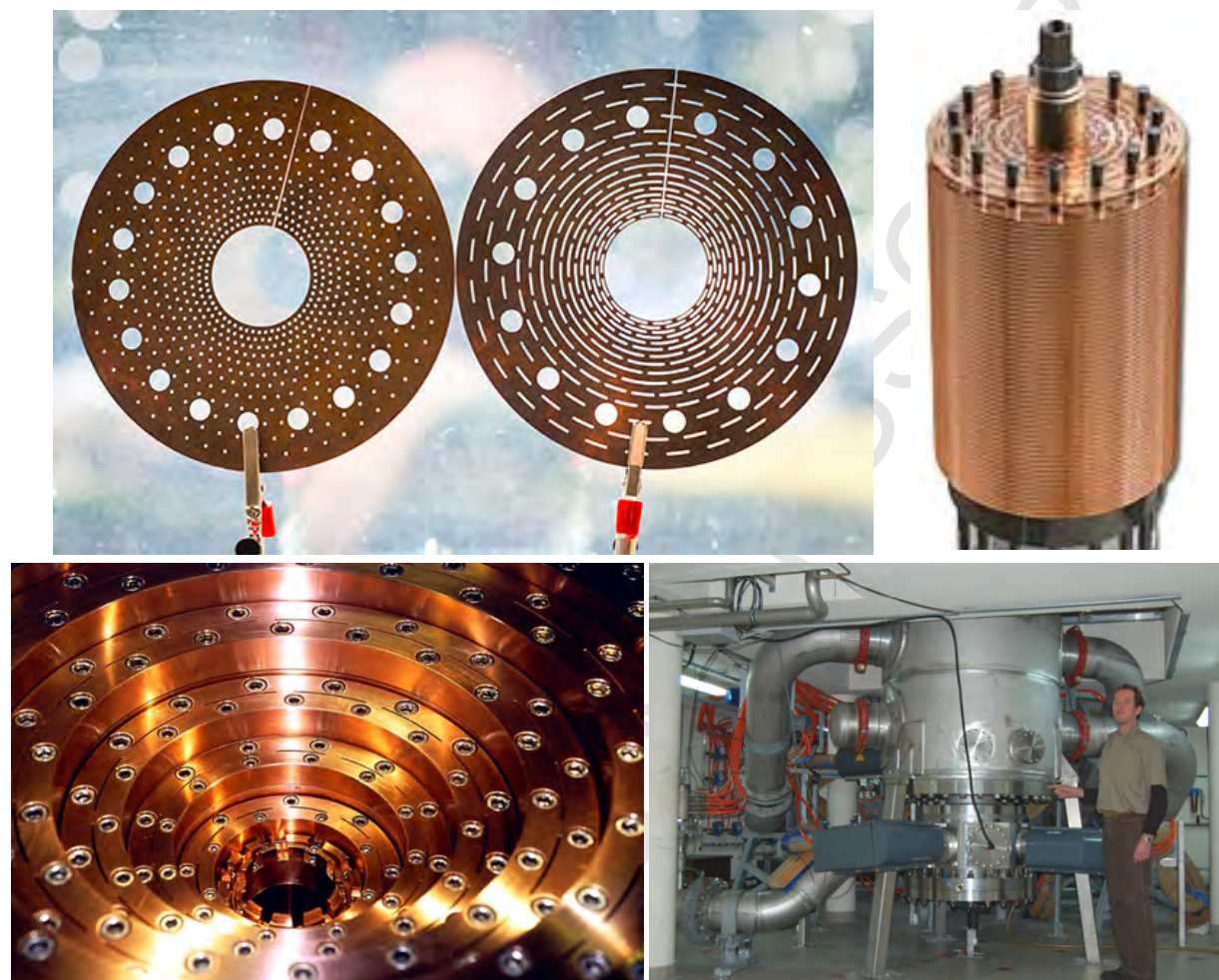
Fig. 19. Top left: Images of the original “Bitter-plate” design (round holes) and the more recent Florida-Bitter-plate design (staggered oval holes), used in the construction of high-field resistive electromagnets. The holes in the plates allow for the efficient flow of cooling water through the magnet, which is needed to dissipate the considerable (10s of MW) resistive heating. The central hole in the plates is about 40 mm in diameter. Top right: these plates, with separating insulating layers, can be stacked in a helical configuration to construct a complete magnet. Photos courtesy NHMFL. Bottom left: top view of a polyhelix assembly used in Grenoble to produce 37 T in a 34 mm bore. Bottom right: the 37 T in 34 mm/24 MW magnet at LNCMI-Grenoble using the polyhelix technology for the inner coils. Photos courtesy CNRS/D. Morel.
