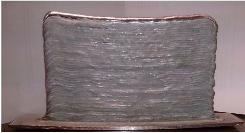
Figure 9. Aluminium wall built with 100 layers deposited using parameter set P5.
