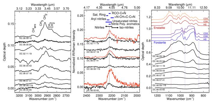
**Fig. 3.** Measured UCAMMs spectra. *Left*: CH stretching mode infrared optical depth. *Centre panel*: μFTIR (red) and Raman (black) close-up spectra in the nitriles region, normalized to the C=C (IR) and G band (Raman) measured intensities. *Right*: baseline corrected silicate infrared optical depth, along with different absorption models for several size distributions of olivine (forsterite) and pyroxene (enstatite) magnesium rich end members (see text for details).
