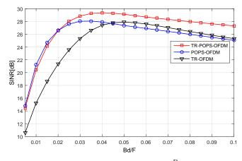
Figure 2: Optimized SINR as a function of  $\frac{B_d}{F}$  for Q = 128, SNR = 30 dB,  $B_d T_m = 10^{-3}$  and D = 3T.
