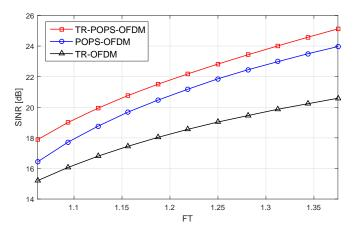
Figure 3: SINR versus FT for Q = 128, SNR = 30 dB,  $B_dT_m = 10^{-2}$  and D = 3T.
