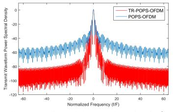
Figure 4: PSD of the optimized transmit waveform for Q = 128, SNR = 30 dB,  $B_dT_m = 10^{-3}$ , FT = 1.25 and D = 3T.
