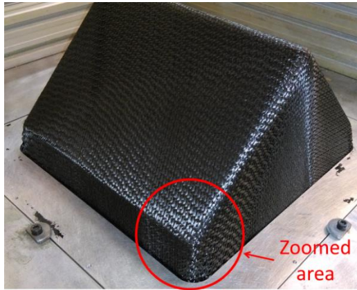
Figure 7 : Quality preform with pressure increasing and adapted blank-holders geometry
