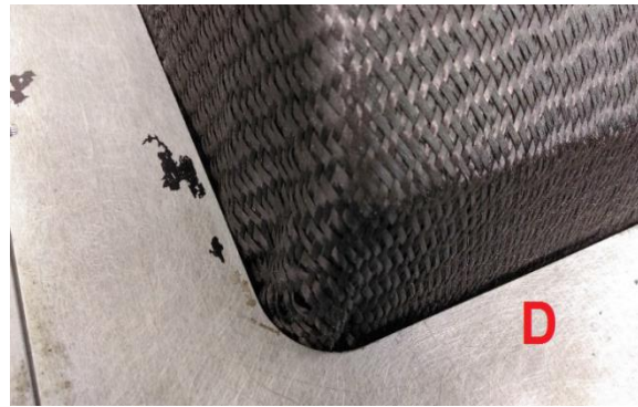
Figure 6 : Quality preform with adapted blank-holders geometry, case of monolayer oriented at 30°
