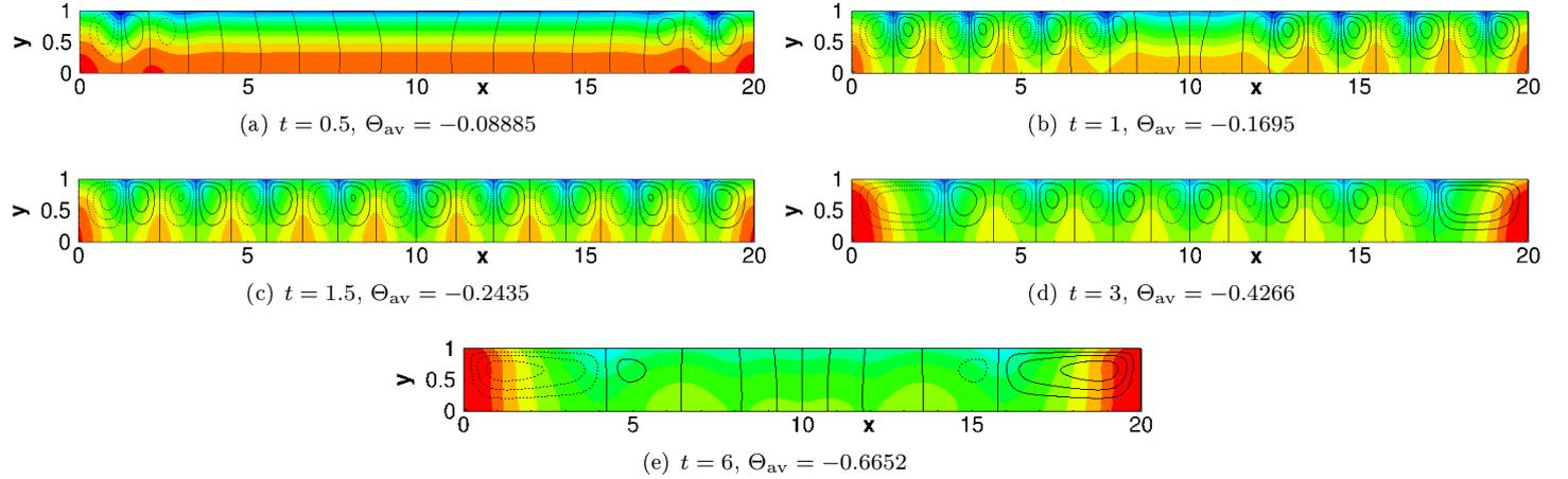
Figure 3: Fluctuation of the temperature field around its average value  $\Theta_{av}(t)$  (coloured field,  $\Theta(x, y; t) - \Theta_{av}(t) \in [-0, 06; 0, 04]$ ) and stream lines for  $e = 1$  mm,  $\mu = 3.25$  mPa  $\cdot$  s,  $h_{side} = 10$  W/(m<sup>2</sup>  $\cdot$  K) and  $r = 0$ .
