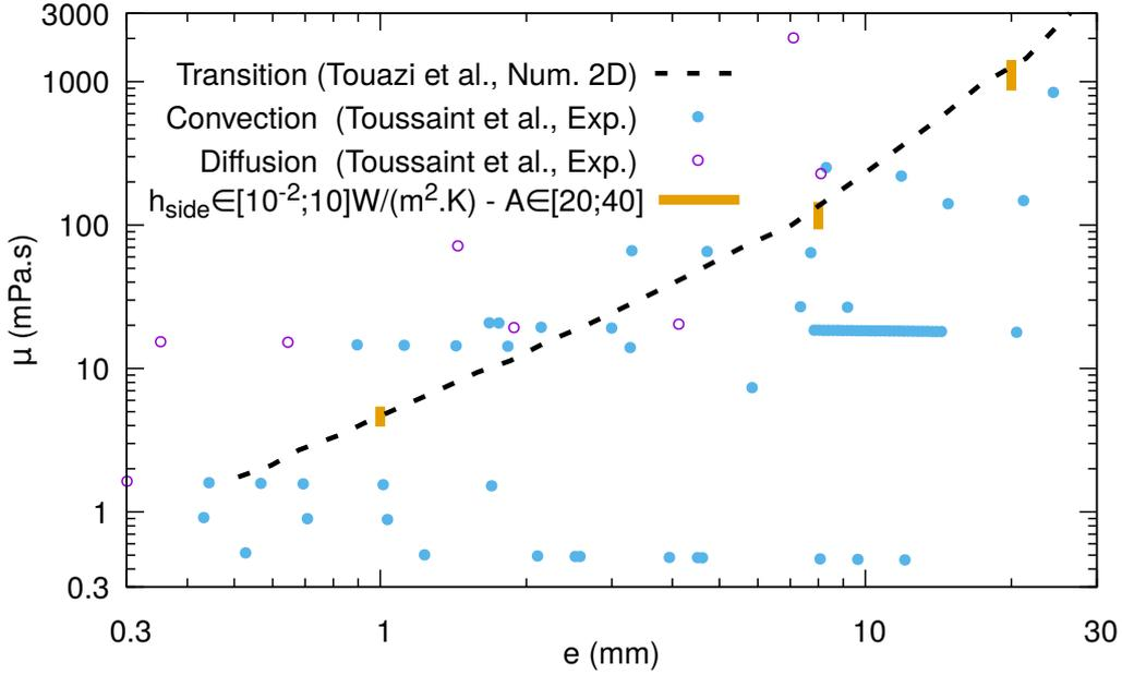
Figure 15: Comparison between the critical viscosity intervals defined for  $h_{\text{side}} \in [0.01; 10] \text{ W}/(\text{m}^2 \cdot \text{K})$ ,  $A \in [20; 40]$ ,  $r = 0$  and three thicknesses ( $e = 1, 8$  and  $20 \text{ mm}$ ), the experimental data by Toussaint et al. [19] and the 2D numerical transition line by Touazi et al. [18].
