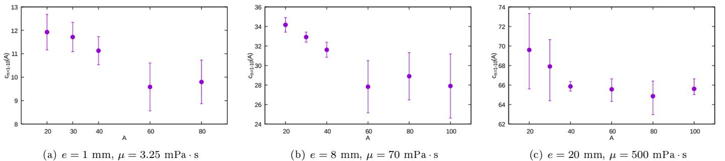
Figure 7: Propagation celerity of the convection wave as a function of the aspect ratio. The vertical bars take into account the different amplitudes  $A_{\text{max}}/2^n$ ,  $n = 1$  to 10, and the filled circle stand for the mean value. Parameters:  $h_{\text{side}} = 10$  W/(m<sup>2</sup>  $\cdot$  K) and  $r = 0$ .
