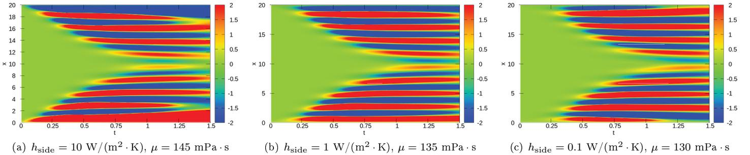
Figure 10: Horizontal velocity at the free surface as a function of time, for  $e = 8 \text{ mm}$ ,  $\mu \lesssim \mu_c$  and  $r = 0$ .
