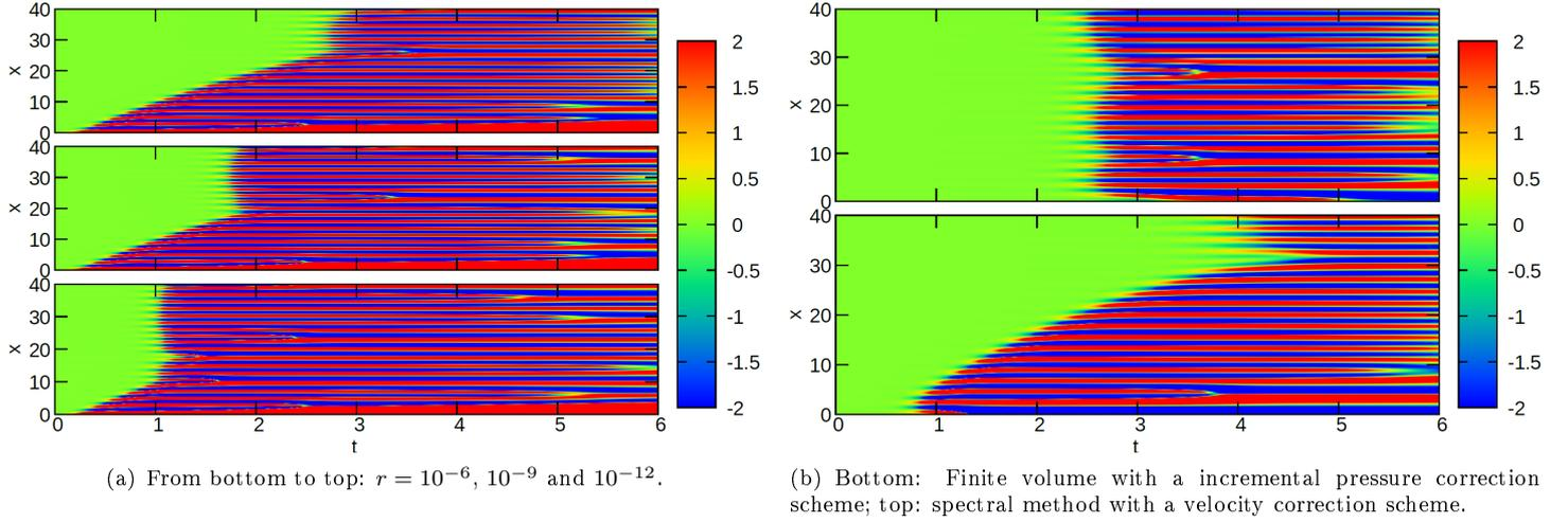
Figure 6: Horizontal velocity at the free surface as a function of time for  $e = 1$  mm,  $\mu = 3.25$  mPa  $\cdot$  s and  $A = 80$ . (a)  $h_{\text{side}} = 10$  W/(m<sup>2</sup>  $\cdot$  K) with different initial temperature perturbations of magnitude  $r$ . (b)  $h_{\text{side}} = 0$  and  $r = 0$  for two incompressible Navier-Stokes solvers.
