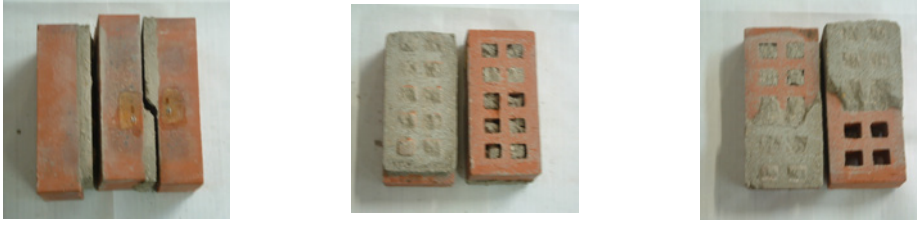
Figure 7. Failure modes - Hollow brick prisms
