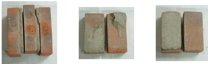
Figure 5. Failure modes - full brick prisms
