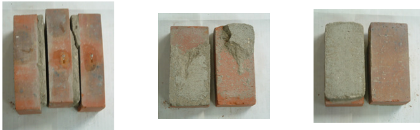
Figure 5. Failure modes - full brick prisms
