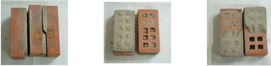
Figure 7. Failure modes - Hollow brick prisms
