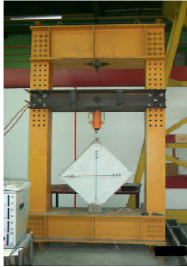
Figure 11. Experimental device for compression diagonal test
