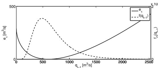
(b) error due to linearisation vs  $q_{t-1}$  distribution.
