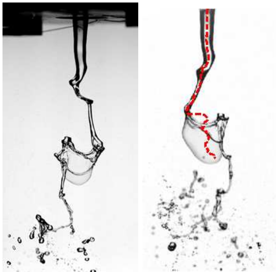
FIG. 4. Left: Typical image of a flapping jet for H_L = 5 mm, H_G = 5 mm, U_L = 0.28 m/s, U_G = 19.5 m/s. Right: Raw image and detected jet center shown in red dashed line.
