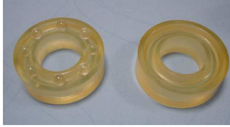
Fig. 4. Ball thrust bearing system made in epoxy
