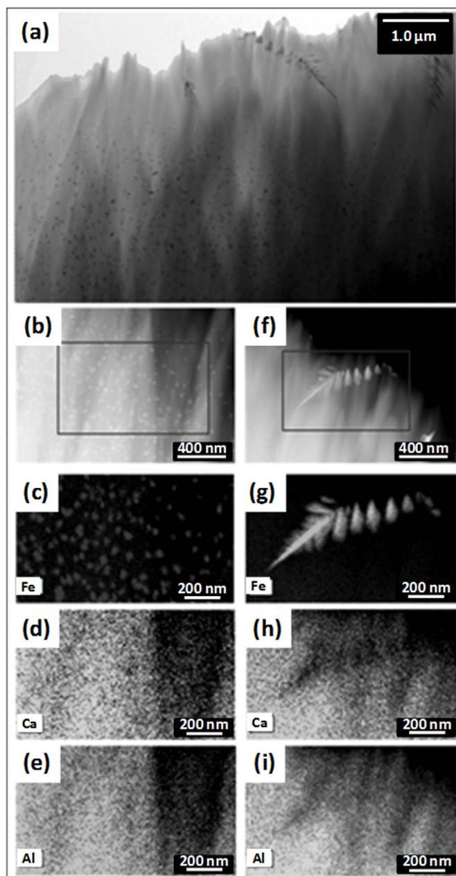
**Figure 3** | Transmission Electronic Microscopy images from a region close to the surface of the OS sample. Two types of crystals were found (star shape and dendritic shape). EDX analyses revealed that Fe is the only cationic element present in these crystals.
