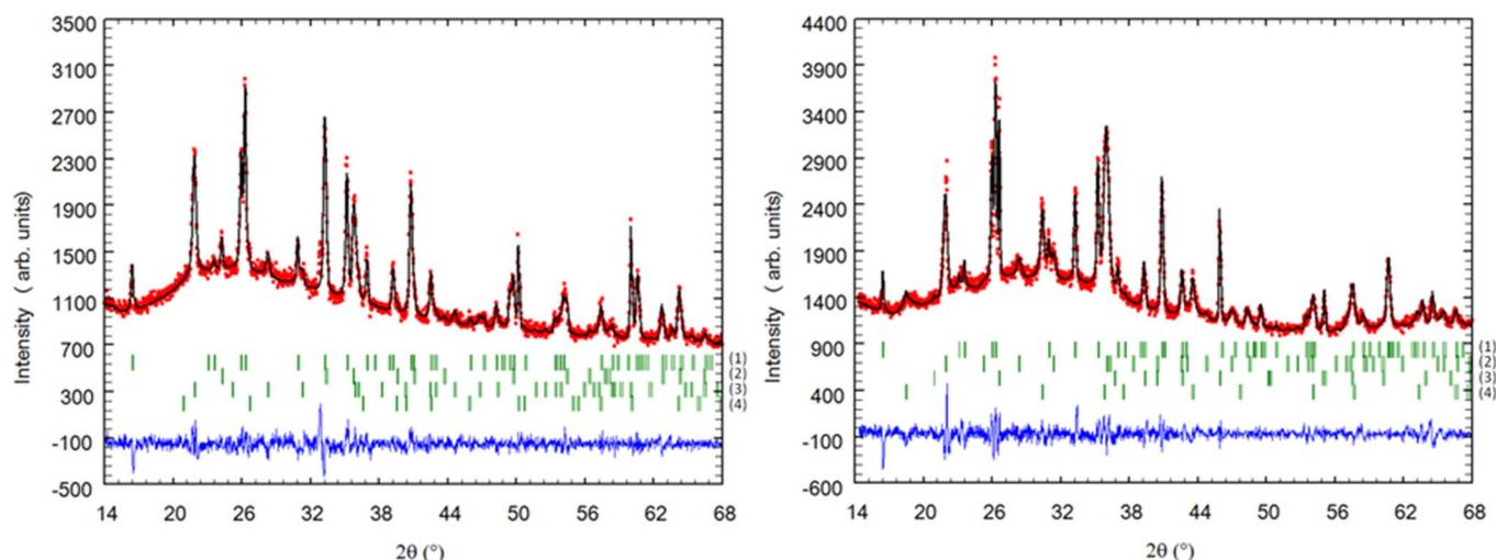
**Figure 6** | Le Bail fitting of the body of the Jian ceramics for the a) HF sample: (1) Mullite, (2) Hematite, (3) Cristobalite, (4) Quartz, and b) OS sample: (1) Mullite, (2) Magnetite, (3) Cristobalite, (4) Quartz. **Red**: experimental points, **Black**: calculated diagram, **Green**: Bragg positions, **Blue**: difference curve.
