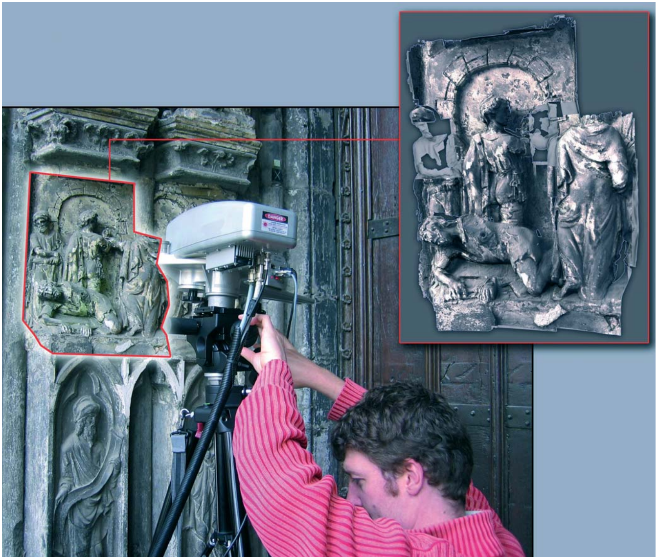
Fig. 7: In situ 3D digitalization of the external sculptures of a portico at the Tournai Cathedral (Belgium) by DEIOS.
