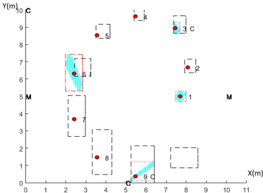
**Fig. 5** Correction step. Hypotheses of the robot poses along the trajectories in  $x$ - $y$  plane (meters): Predicted hypothesis is represented by dashed rectangle, Corrected hypothesis by dotted rectangle and new hypothesis by dashed-dot rectangle.
