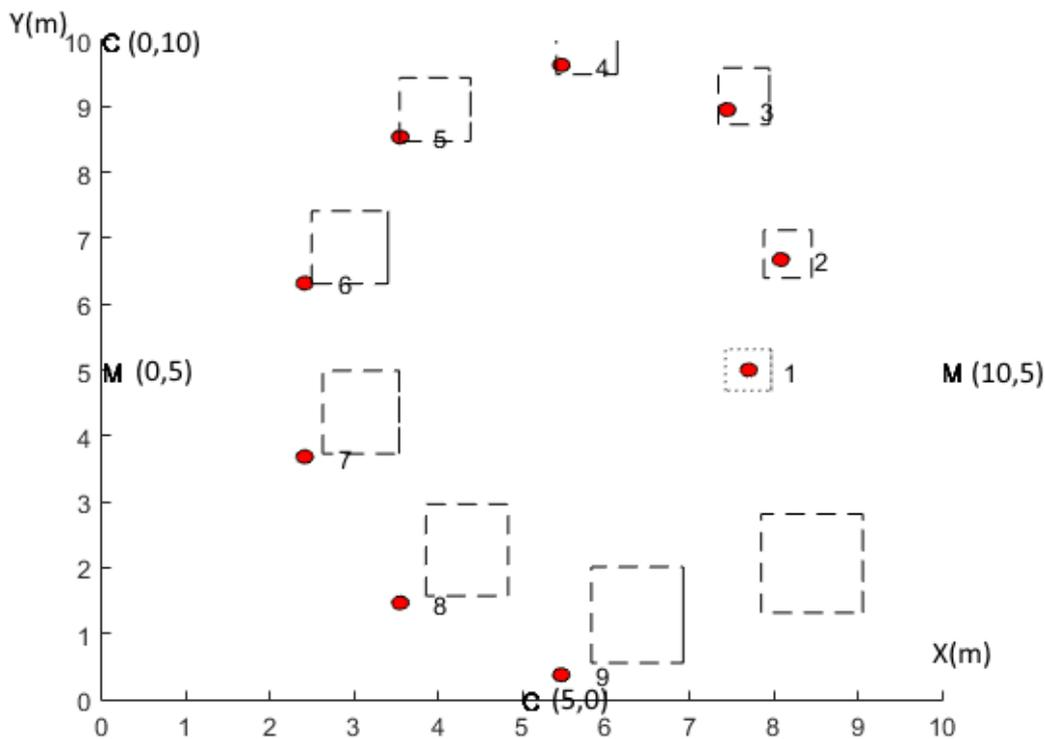
**Fig. 3** Predicted step. Predicted hypotheses (dashed rectangle) of the robot poses along the trajectories in x-y plane (meters). Labels C and M respectively stand for goniometric sensor and marker. Labels are located at the device coordinates. True robot position is represented by a large point
