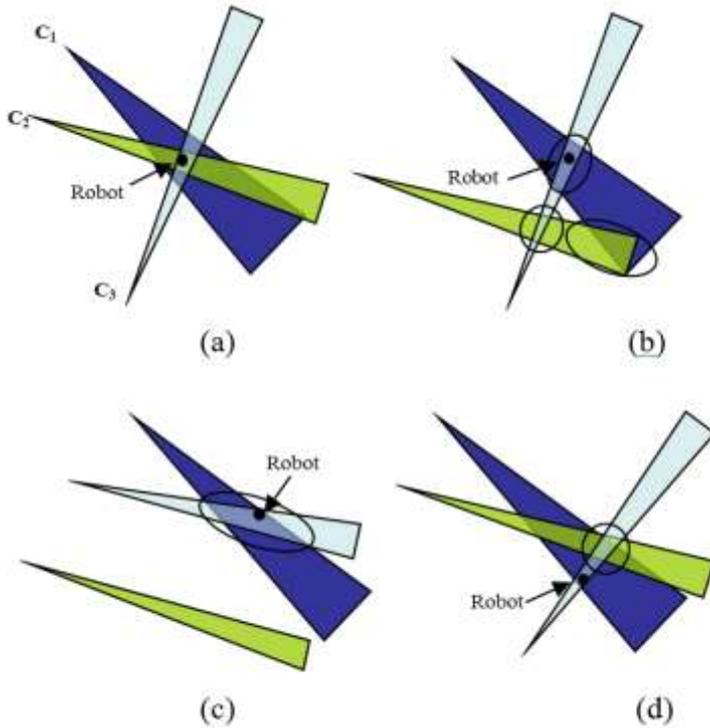
**Fig. 2** Outlier processing. **a** No inconsistent measurement. **b** One detectable inconsistent measurement, **c** One detectable and identifiable inconsistent measurement. **d** No detectable inconsistent measurement, the true robot localization is not in the intersection area of the three measurements
