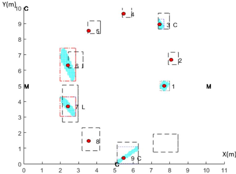
**Fig. 7** BEES algorithm. Hypotheses of the robot poses along the trajectories in x-y plane (meters): Predicted hypothesis by dashed rectangle, Corrected hypothesis by dotted rectangle and new hypothesis by dashed-dot rectangle. Labels C and M respectively stand for goniometric sensor and marker. Labels are located at the device coordinates. True robot position is represented by a large point
