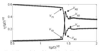
**Fig. 4.** Time evolution of the particle velocities (same case as in Fig. 3) during the bouncing of two spheres. The terminal velocity  $V_{Ti}$  and rebound velocities  $V_{Ri}$  and  $V_{Si}$  of particle i are represented.
