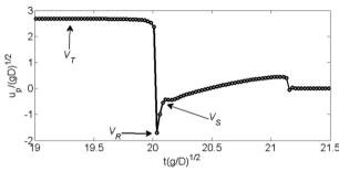
**Fig. 2.** Time evolution of the sphere velocity (same case as in Fig. 1). The terminal velocity  $V_T$  and the rebound velocities  $V_R$  and  $V_S$  are represented.
