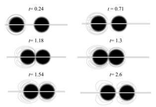
**Fig. 3.** Iso-vorticity contours from -4.25 to 4.25 over time of two spheres bouncing with  $\rho_p/\rho=8$ , St=140 and  $Re\approx175$ . Positive (resp. negative) values are continuous (resp. dashed) lines. Images are mirrored. The particle on the left (right) is labelled particle 1 (2).
