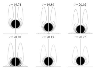
Fig. 1. Iso-vorticity contours from -17.8 to 17.8 of a sphere bouncing on a wall with with  $\rho_p/\rho=8$ , St=53 and  $Re\approx60$ . Positive (resp. negative) values are continuous (resp. dashed) lines. Images are inspired from [11] and have been mirrored.
